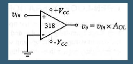
$$+V_{sat} = +V_{CC} - 2$$
